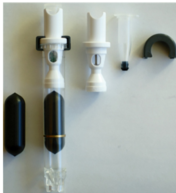
Figure 1 Components of the AccuCyte ® system. From left to right is pictured the float; the entire assembly for separation and isolation of the buffy coat, including the Separation Tube with sealing ring; the EpiCollector ® ; the Transfer Tube with septum base that is pierced by the EpiCollector needle to allow the flow of material from the Separation Tube to the Transfer Tube; and the clamp that secures the entire apparatus.
