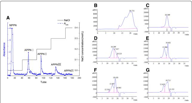
**Fig. 1 a** Elution curve of CPPN via DEAE Sepharose Fast Flow anion exchange chromatography column. **b** High performance gel permeation chromatogram of CPPN. **c** High performance gel permeation chromatogram of NPPN. **d** High performance gel permeation chromatogram of APPNII. **e** High performance gel permeation chromatogram of APPNII. **g** High performance gel permeation chromatogram of APPNIII. **g** High performance gel permeation chromatogram of APPNIII.
